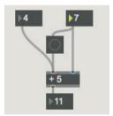
Fig. IA.3 How to make a "cold" inlet behave like a "hot" one
