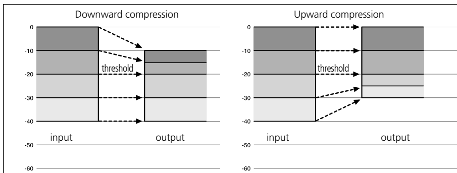
fig. 7.1: downward e upward compression 5
