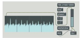
Fig. 5.3 Making a glissando with a non-bandlimited waveform
