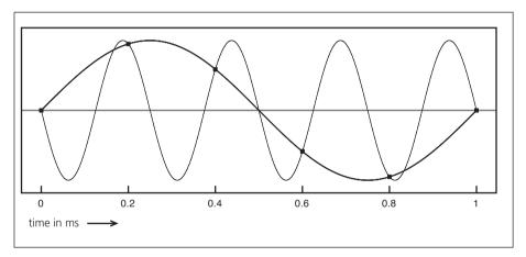
Fig. 5.8 Two sine waves with frequencies of 1000 Hz and -4000 Hz sampled at a rate of 5000 Hz.
