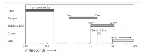
Fig. 6.1 Different delay times from filters to echoes
