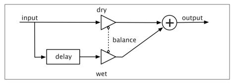
Fig. 6.2 A simple delay example
