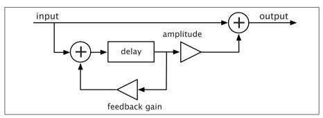
Fig. 6.3 Block diagram for delay with feedback
