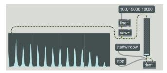
Fig. 5.4 The spectrum of a bandlimited waveform
