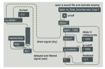
Fig. 6.7 "Tape Delay" with lowpass filter and feedback
