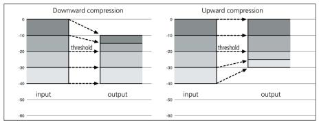
Fig. 7.1 Downward and upward compression<sup>5</sup>
