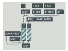
Fig. 6.2 Specifying the delay time with different time formats
