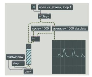
Fig. 7.2 Envelope applied to an oscillator
