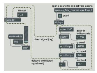
Fig. 6.8 Adding a highpass filter to the tape delay
