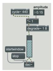
Fig. 5.5 Generating an 8-bit sound
