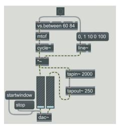
Fig. 6.3 The tapin~ and tapout~ objects
