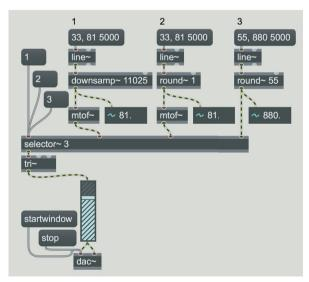
Fig. 8.1 Three different ways to quantize a glissando
