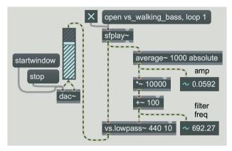
Fig. 7.3 Envelope controlling a filter
