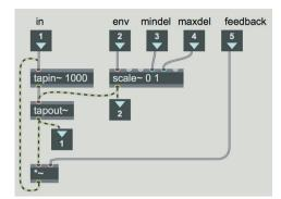
Fig. 7.5 The [p delay] subpatch
