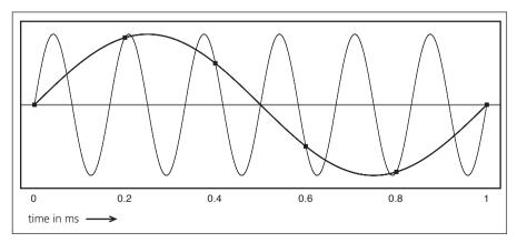
Fig. 5.7 Two sine waves with frequencies of 1000 Hz and 6000 Hz sampled at a rate of 5000 Hz.
